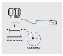
2. Grub screw to tighten between module & module holder and connect module to driver.
