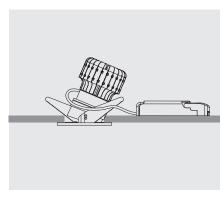
4. Adjust the angle required. Installation complete.
